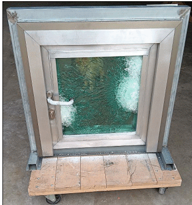
Post Test Sample 1 Rear Side: ZIA-BR-S-FO-98 - Open Out Single Door - NIJ III (.30 cal. 7.62 NATO) - 792 x 736 x 148 mm
